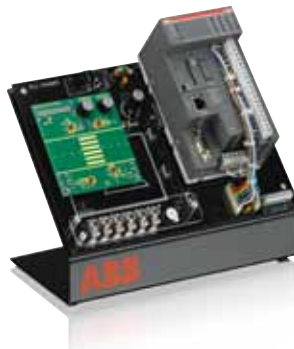
PLC-trainer ABB AC500 with plug-on traffic light module
