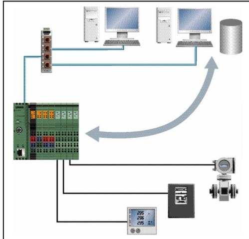
**UDP:** Wireless messages (broadcasts) can be received from other Ethernet devices in the PLC program with UDP. This is done with the same function modules as with TCP/IP.
